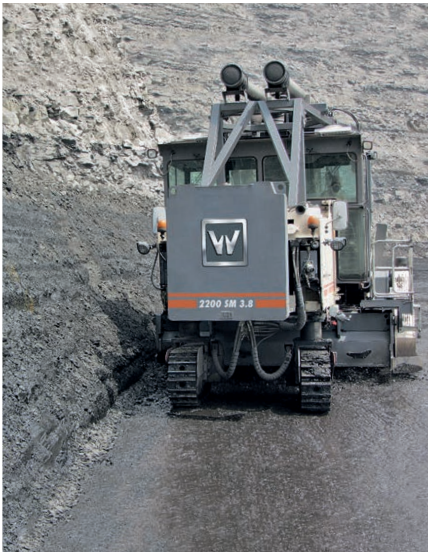
A cutting width of 3.8 m and cutting depth of up to 350 mm guarantee high mining volumes.
