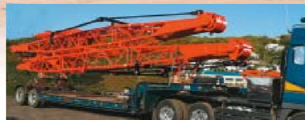
Unitized transport of luffing posts Front and rear posts, along with a set of attachments, are unitized for easier transport.
