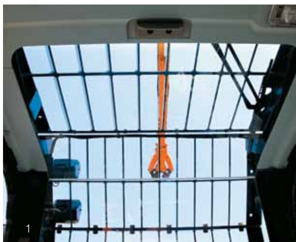
1 Roof window wiper and pillar-less window
