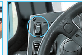
Screen Changeover Switch
