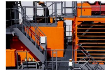
This area is conveniently located at the center of the body and provides access to the engine as well as the hydraulic and electrical systems.
