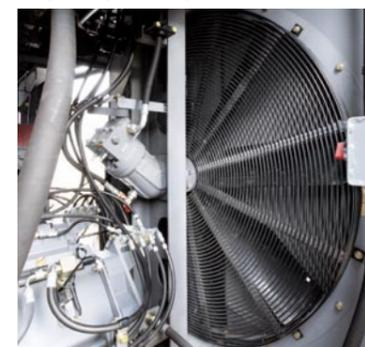
The oil cooler is used for optimal cooling efficiency. It is positioned far from the engine radiator for even better cooling potential.
