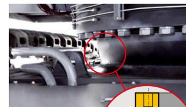
The center track frame of integral cast steel structure can avoid stress concentration, and increase reliability.
