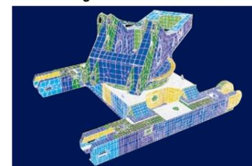
Computer-assisted analysis was used to check that the frame box can withstand heavy-duty excavation work.
