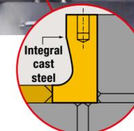
**Rugged Track Links—** Shoes include roller guides for extended service life.
