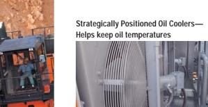
Four oil coolers are used for optimal cooling efficiency. They are positioned far from the engine radiator for even better cooling potential.
