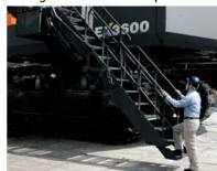
Folding stairs is designed for easy access to the machine for servicing and maintenance.
