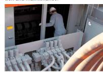
This area is conveniently located at the center of the body and provides access to the engine as well as the hydraulic and electrical systems.
