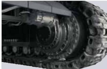
This design helps protect the travel motors from damage by rocks.
