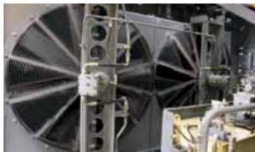
Two oil coolers are used for optimal cooling efficiency. They are positioned far from the engine radiators for even better cooling potential.
