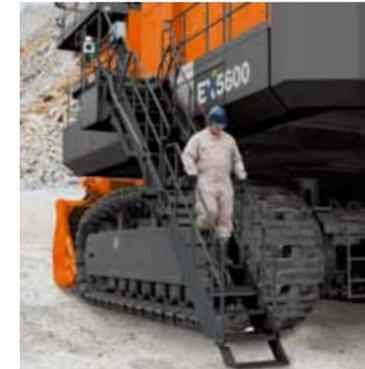
Folding stairs are designed for easy access to the machine for servicing and maintenance.
