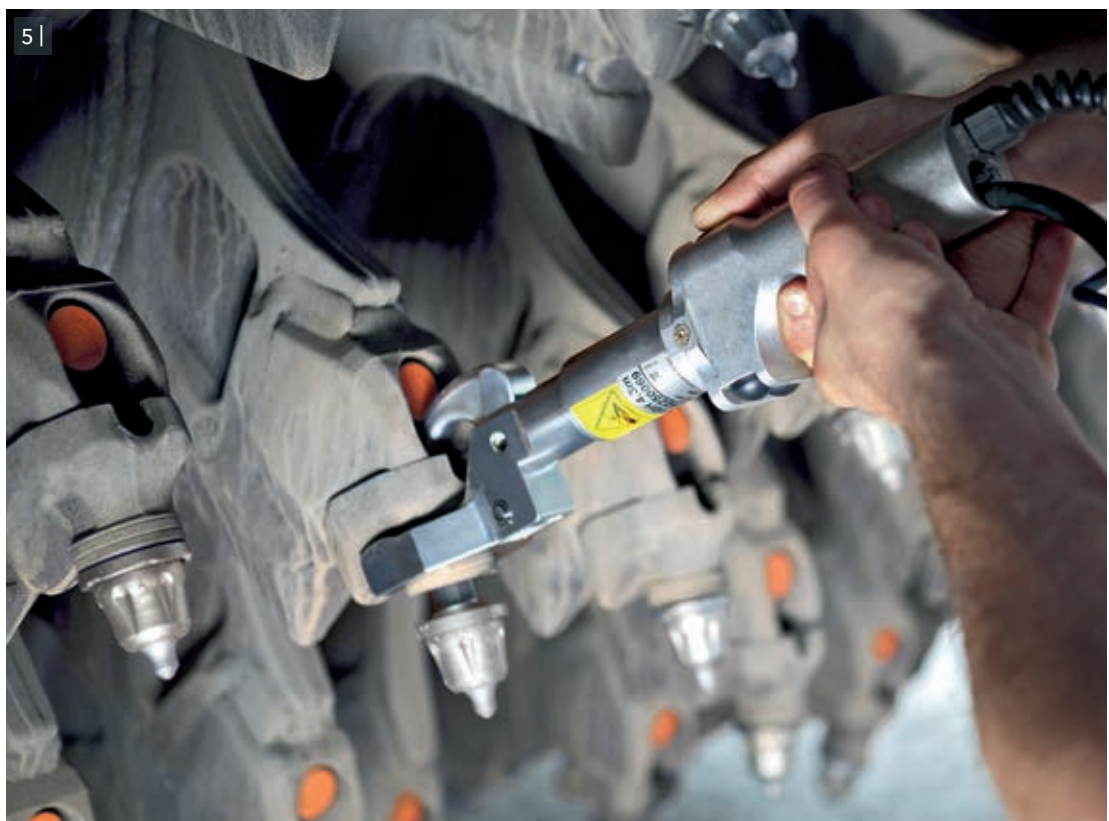
5 | Tool replacement made easy using the hydraulic cutting tool extractor.
