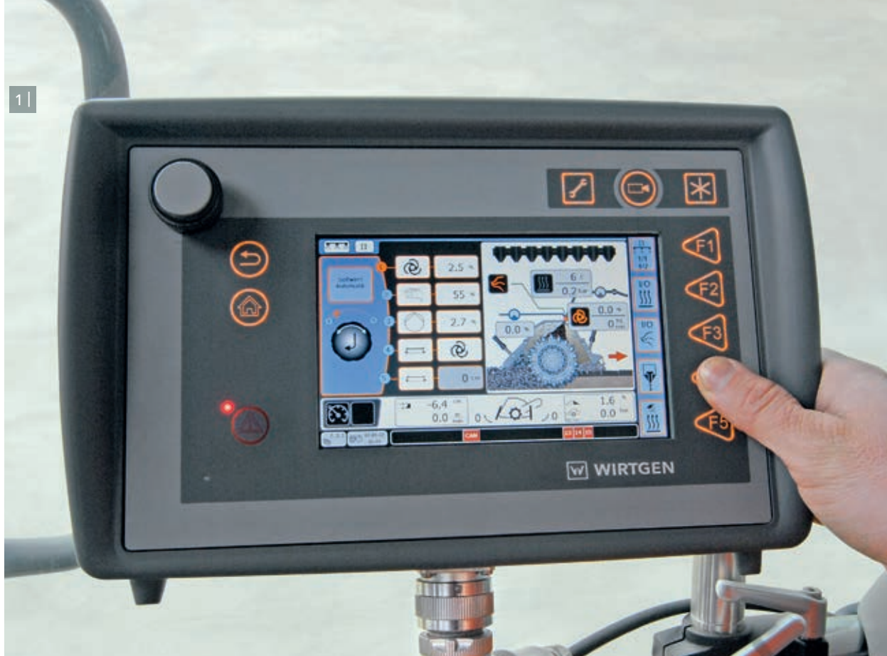
1 | At a glance: important machine parameters are permanently displayed in the bottom menu bar of the metering menu.
