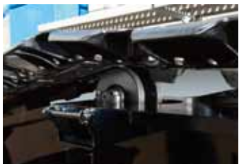
Four upper rollers Hydraulic shoe tension device OPTION
