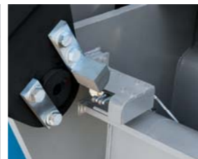
Secondary boom hoist limiting device that cannot be released by the operator
