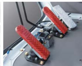
Winch with free fall function (brake pedals)
