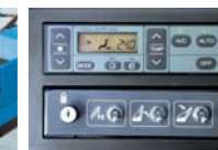
Full auto air-conditioner (with heater and cooler box, uses substitute chlorofluorocarbon)
