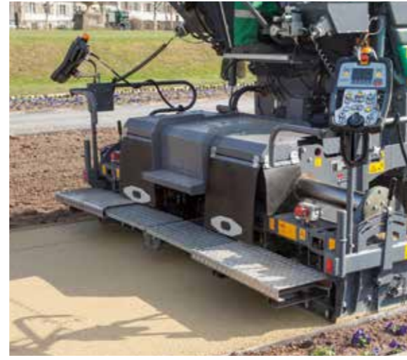
AB 340 V built up with 25cm bolt-on extensions
