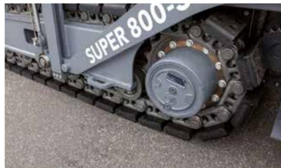
» **Thanks to powerful separate drives** fitted into the sprockets of the crawler tracks, engine output is translated into pave speed with no loss of power.
