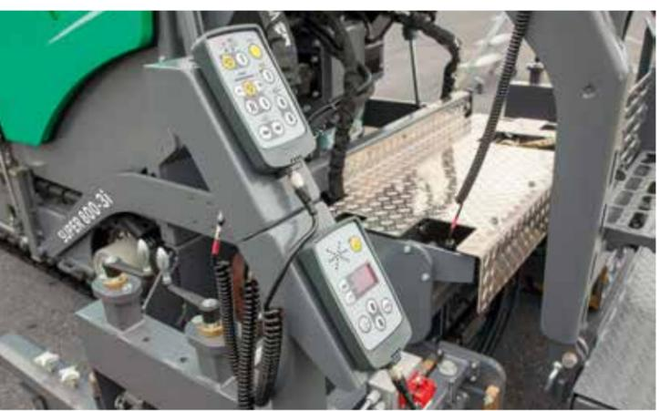
The **ErgoBasic operating concept** was developed on the basis of the proven ErgoPlus operating system which is installed in VÖGELE's large pavers, but it was tailored specifically to the needs and requirements of the users of our Mini Class pavers.
