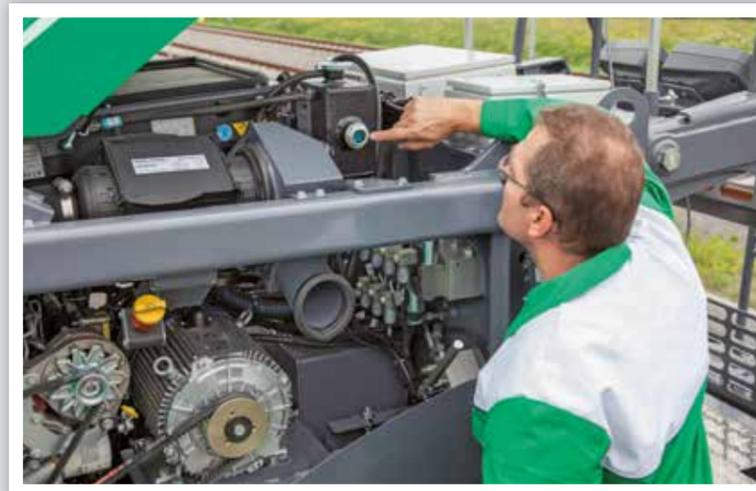
**The standardized service concept** conceived for the VÖGELE pavers means that servicing is quick and uncomplicated. Large hinged panels provide convenient access to all service points on the machine.
