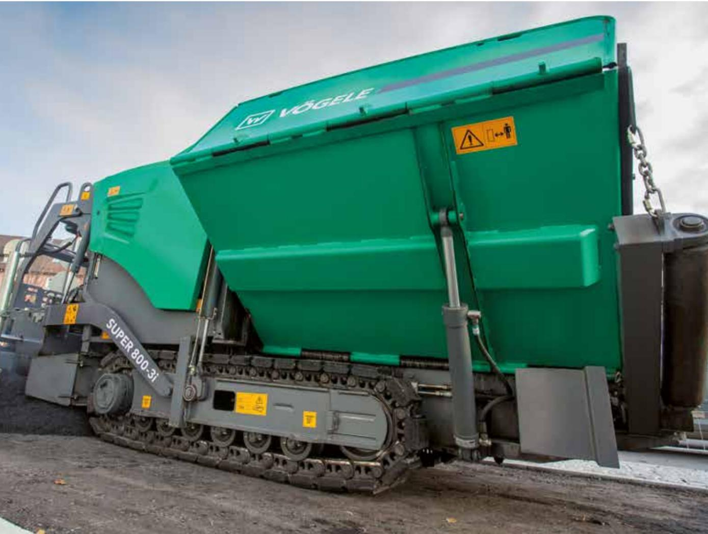
**Positive tracking** when moving straight and accurate cornering due to separate drive and electronic control provided for each crawler track.
