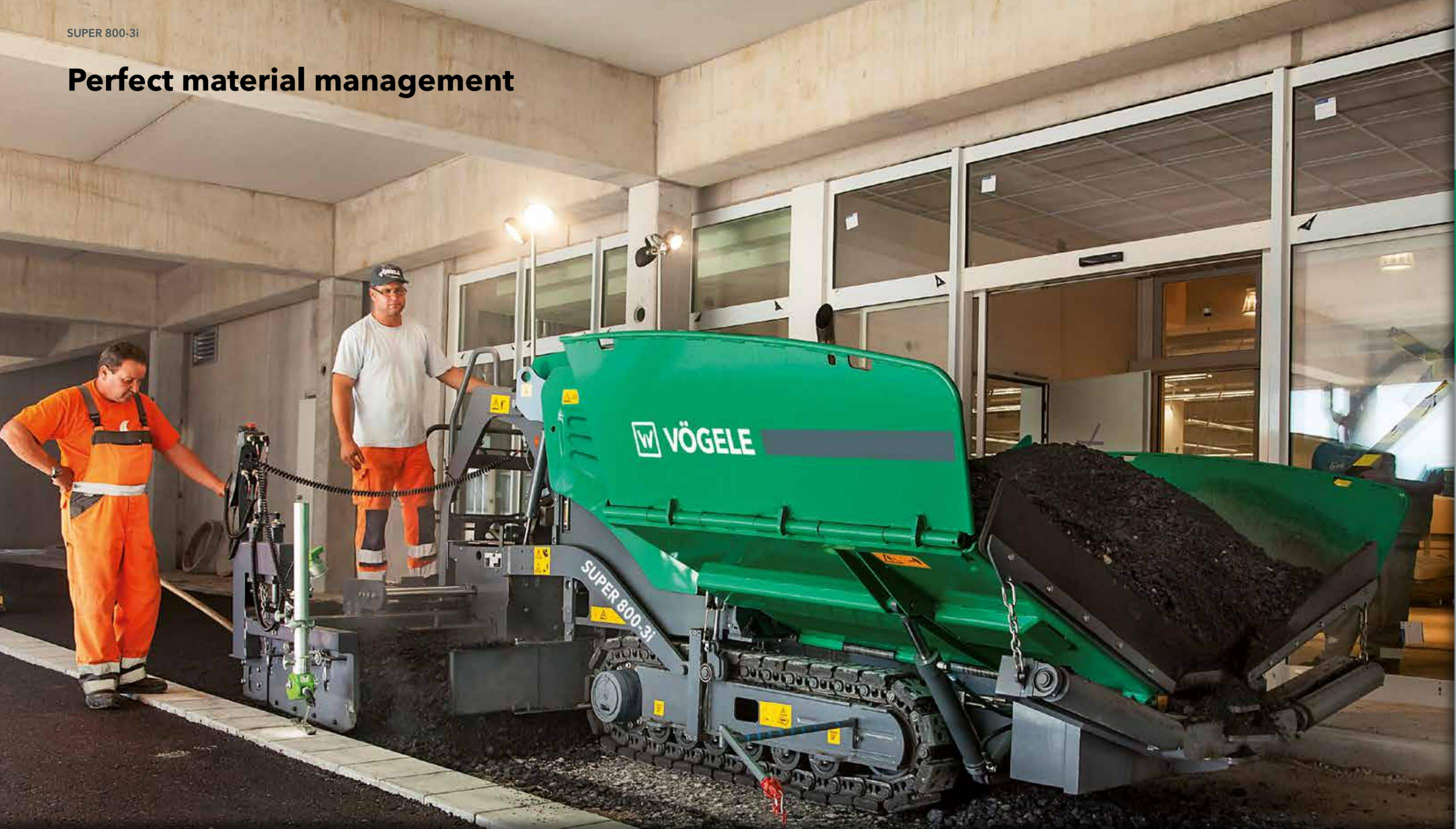
**Several feeding options** are particularly useful when space is narrow and confined. That is exactly what the large material hopper of the SUPER 800-3i was designed for. It can be conveniently supplied with material by lorry or wheeled loader, depending on how much space is available.
