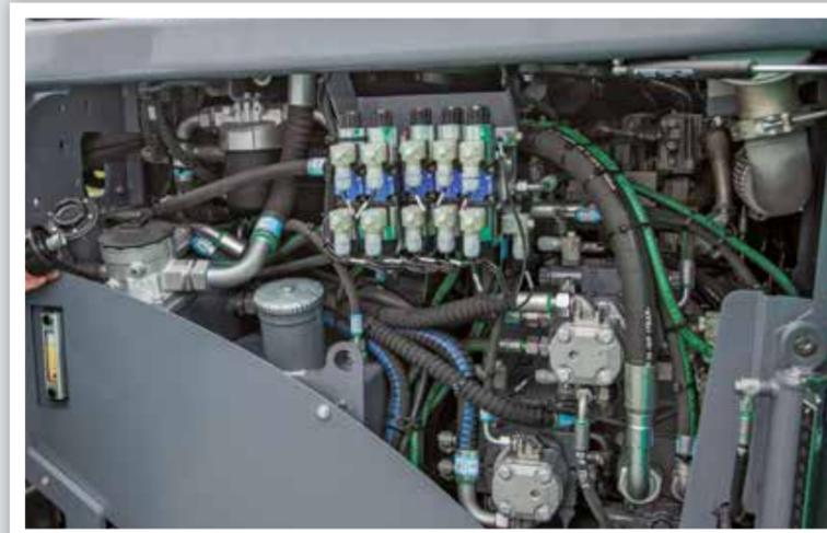
**All hydraulic pumps** are located on the splitter gearbox and provide maximum service-friendliness thanks to their clear arrangement and easy accessibility.
