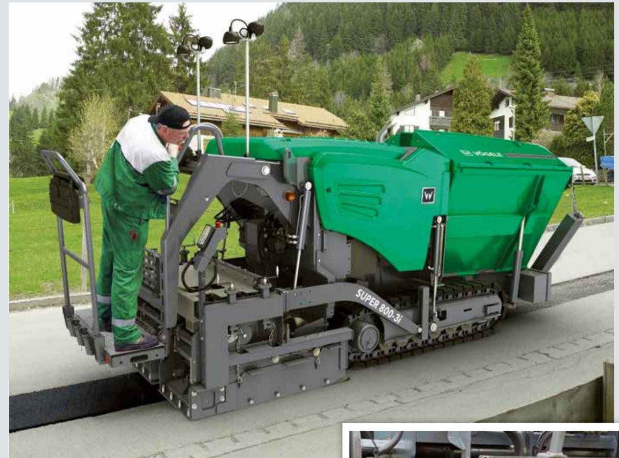
*With the system for pave width reduction fitted, the screed floats on the mix just as it does when paving in a non-reduced width. This allows the layer thickness to be adjusted via the screed tow point rams or even to be controlled with Niveltronic Basic.*
