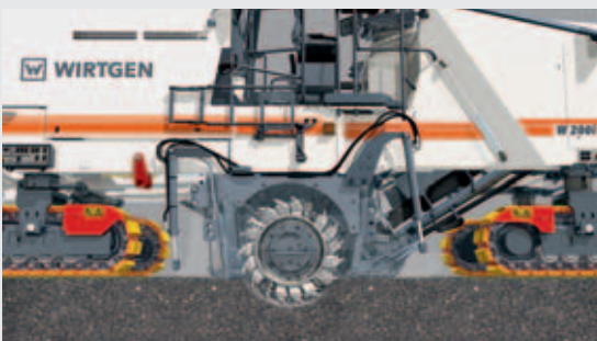
3 | The milling machine is lowered slowly while retaining its parallel alignment
