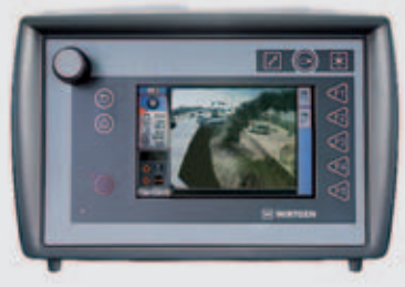
2 | Camera at end of conveyor
