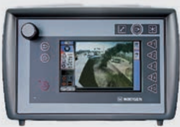
2 | Camera at end of conveyor
