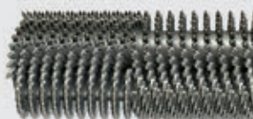
Micro-fine milling drum Milling width: 2,000 mm Milling depth: 0-30 mm Tool spacing: 6 x 2 mm
