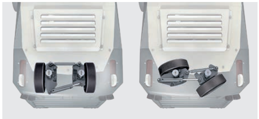
The front axle enables large steering angles.
