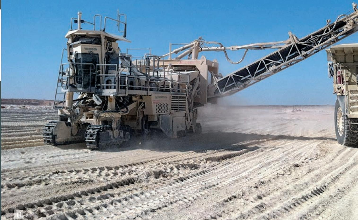
1 | *The high-capacity discharge conveyor can be slewed about 90° to the left...*
