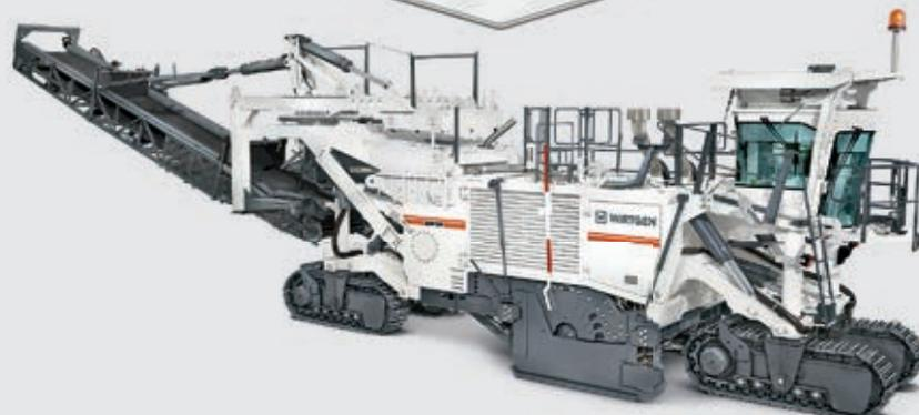
*A single operation instead of four - with the WIRTGEN 2500 SM surface miner.*
