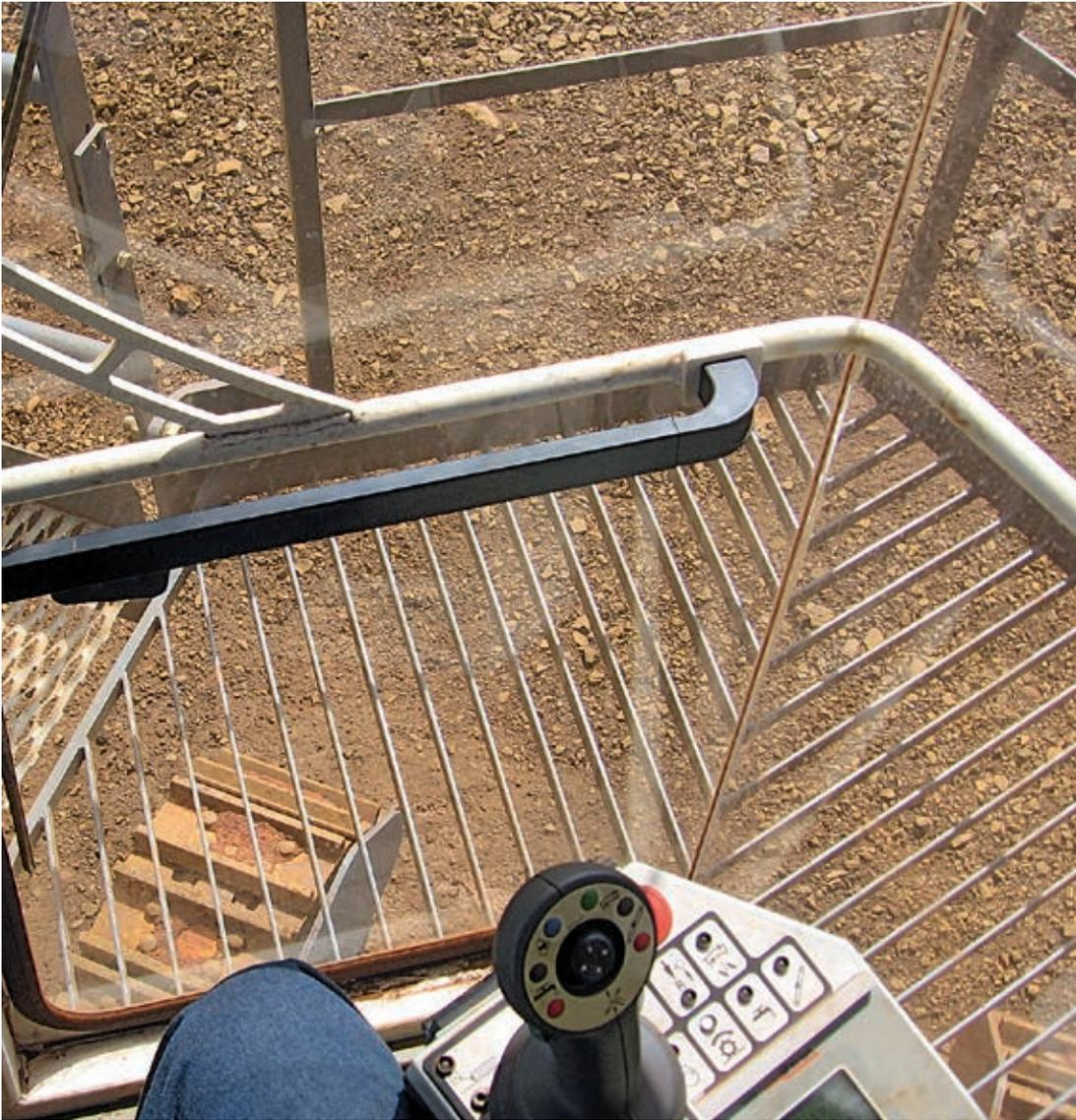
*The operator's cab offers a perfect view of the space between the front track units ...*
