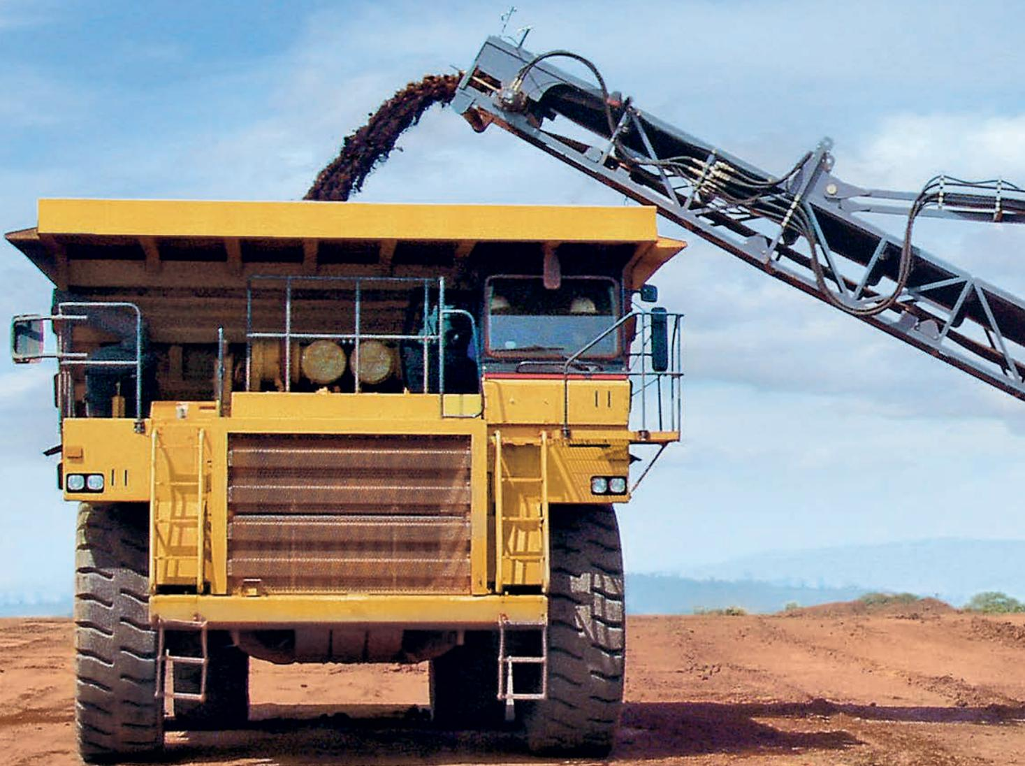
A BIG IDEA. MINING VALUABLE USEFUL MINERALS SELECTIVELY NOT IN FOUR WORK STEPS BUT IN A SINGLE OPERATION. WITH THE WIRTGEN 2500 SM. A HIGH-PERFORMANCE SURFACE MINER IN HEAVY-DUTY DESIGN FOR RELIABLE, CONTINUOUS OPERATION AROUND THE CLOCK. EQUIPPED WITH OUR EXPERTISE IN STATE-OF-THE-ART CUTTING TECHNOLOGY. WITHOUT DRILLING AND BLASTING BUT IN A HIGHLY ENVIRONMENTALLY GENTLE PROCESS YIELDING MATERIAL OF THE PUR-EST QUALITY. WIRTGEN SURFACE MINING - EXPLOITING MINERAL DEPOSITS THE INTELLIGENT WAY.
