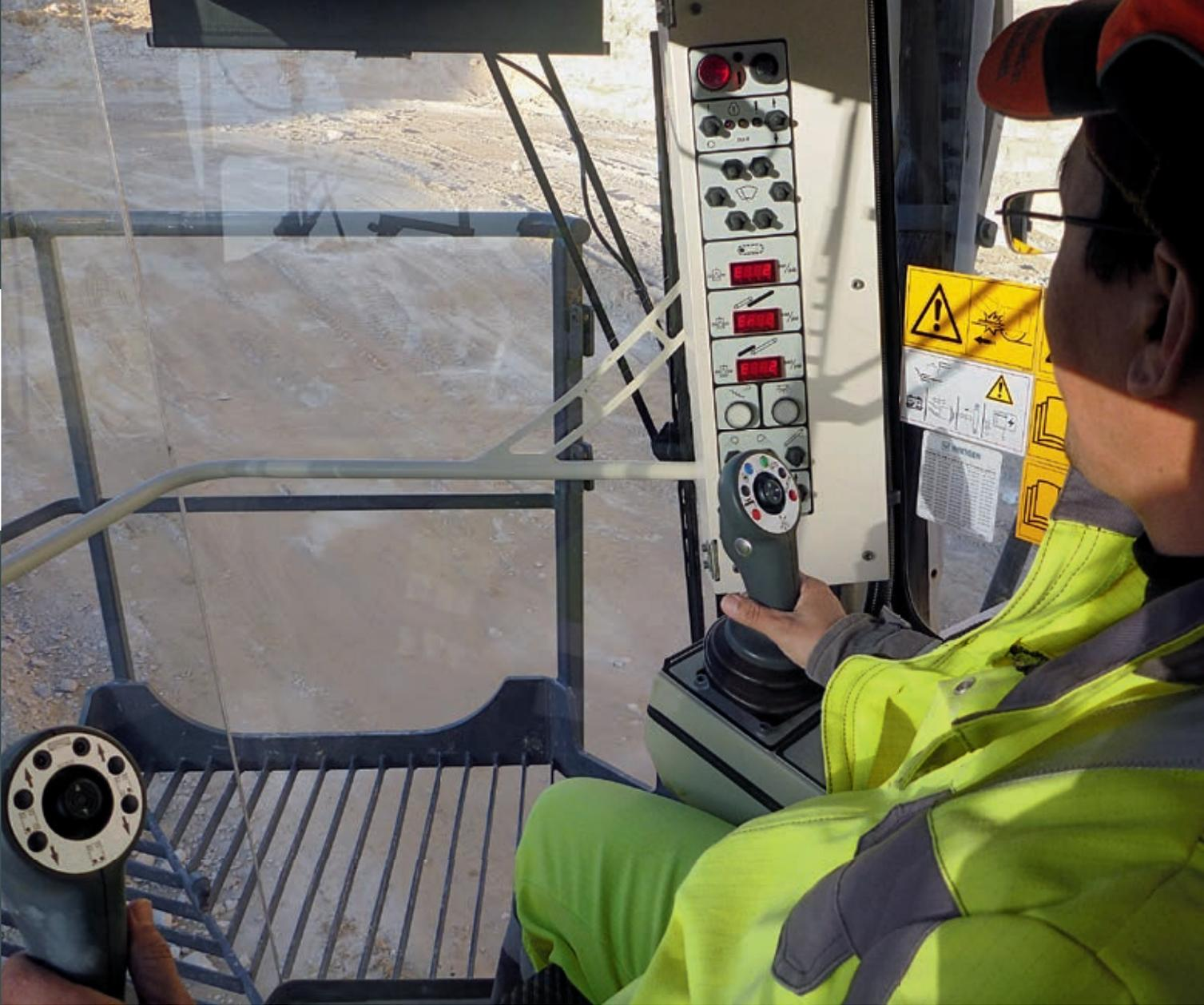
*Operation of the 2500 SM is simple and logical via two multifunctional joysticks integrated in the armrests.*
