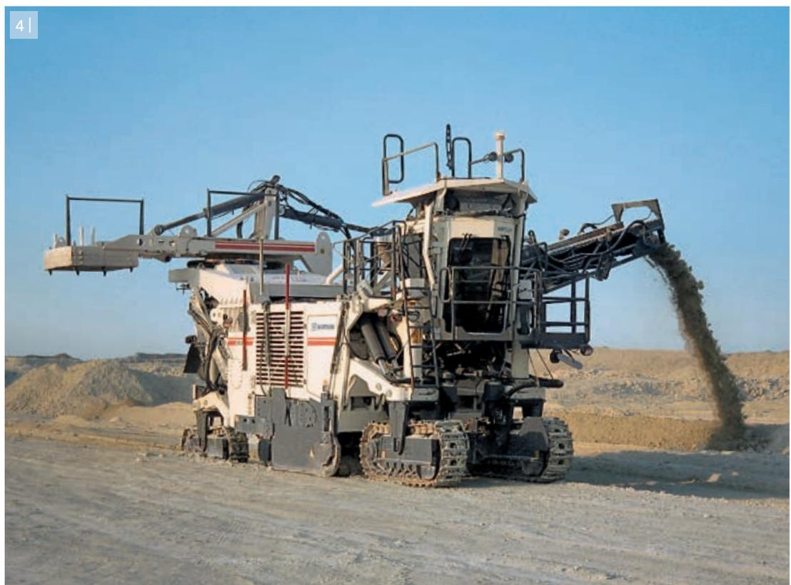
4 | The counterweight provides stability, for example, when discharging the mined material to the side of the machine.
