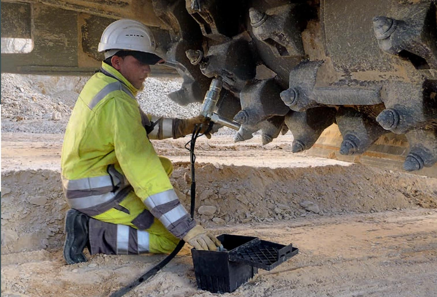
*The hydraulically operated tool extractor ensures the quick and effortless replacement of cutting tools.*
