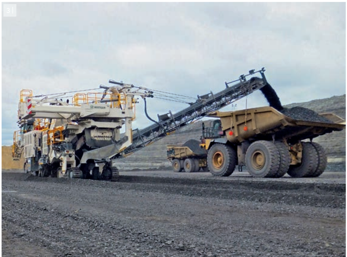
2 | Extracted material can also be simply discharged to the side of the miner.
