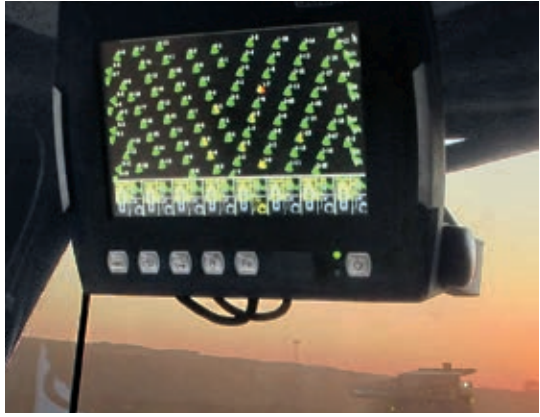
Worn tools are identified by means of an optical measuring process and then marked in colour on a screen.
