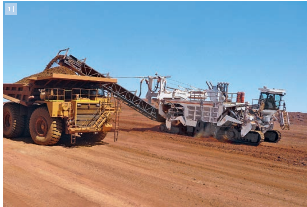
1 | Slewing angles of up to 90° to either side allow perfect adjustment to conditions in the mine.
