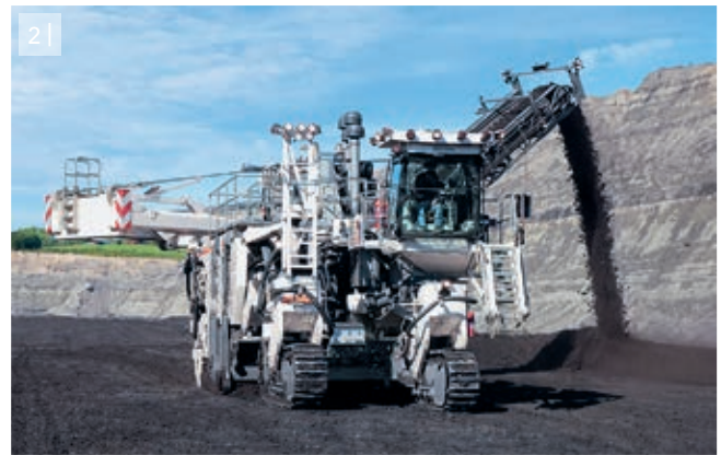
1 | Slewing angles of up to 90° to either side allow perfect adjustment to conditions in the mine.
