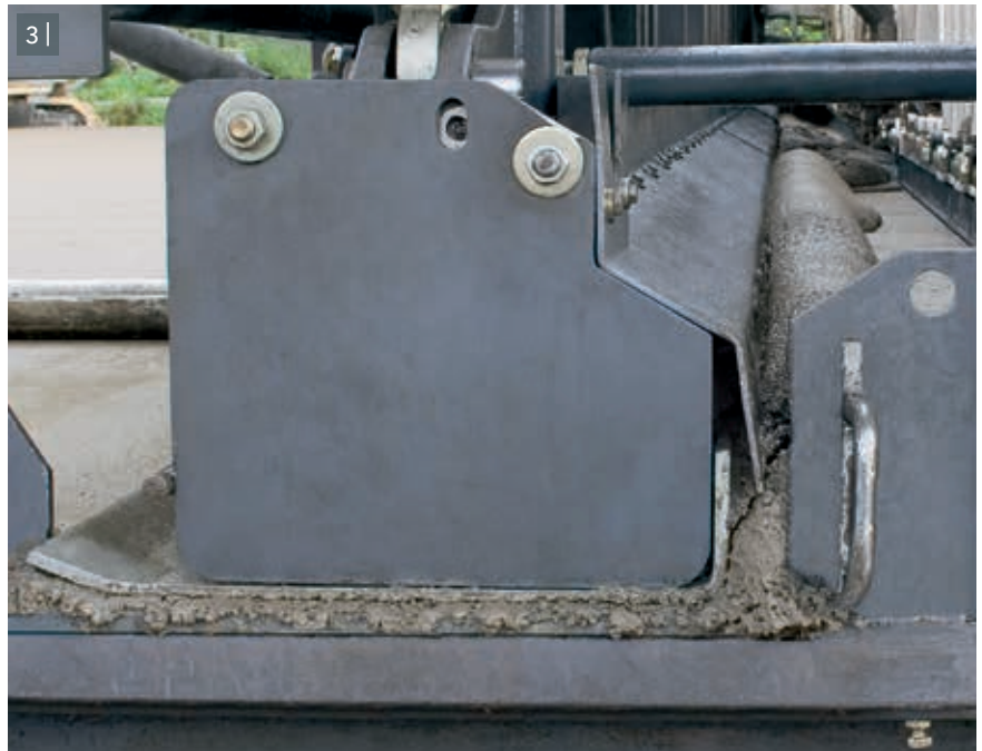
3 | The heavy-duty oscillating beam produces an even surface.
