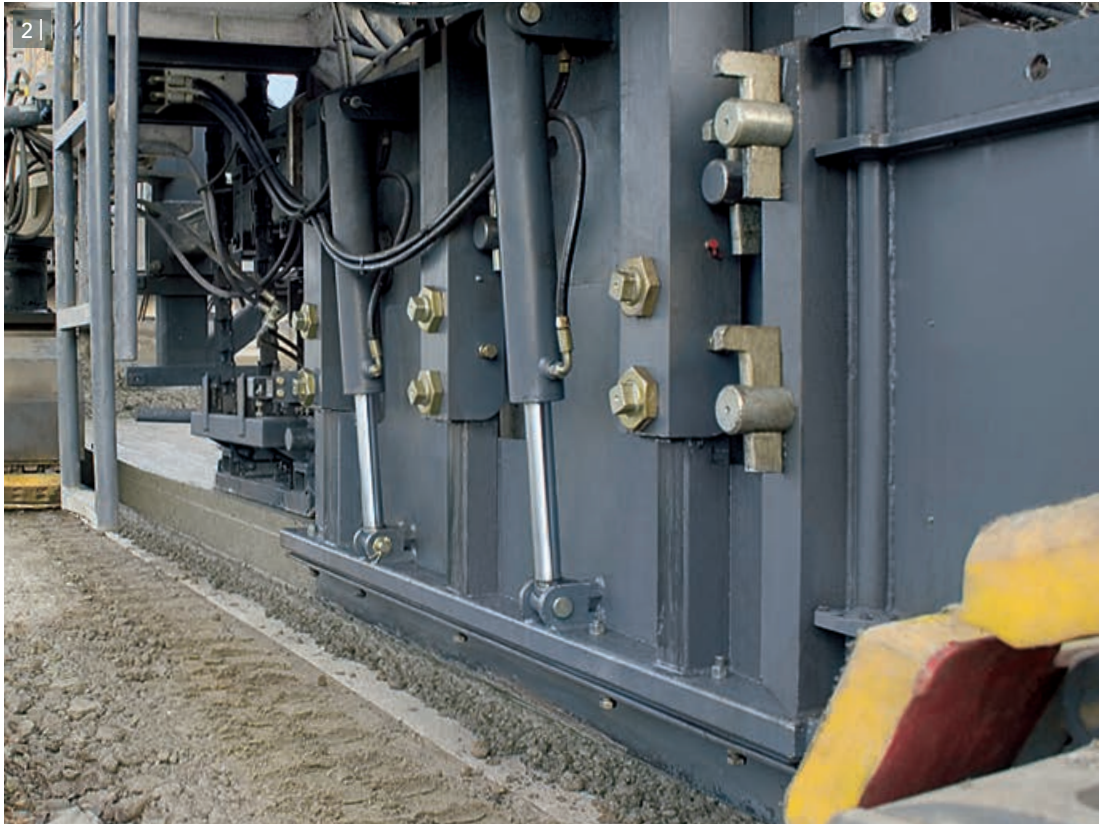
2 | Hydraulically adjustable side-plates ensure clean concrete edges.
