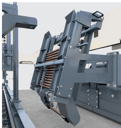
Longitudinal joint tie bar inserter (SP 94/SP 94i only).
