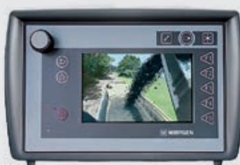
2 | Camera at end of conveyor
