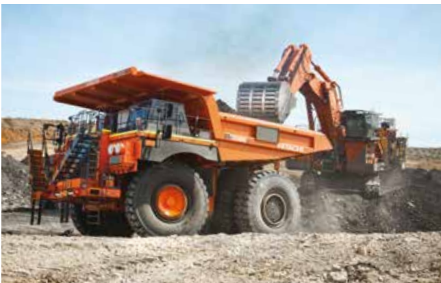
EH dump trucks and EX ultra-large excavators
