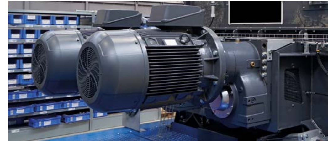
Mechanical and electric test run at the factory
