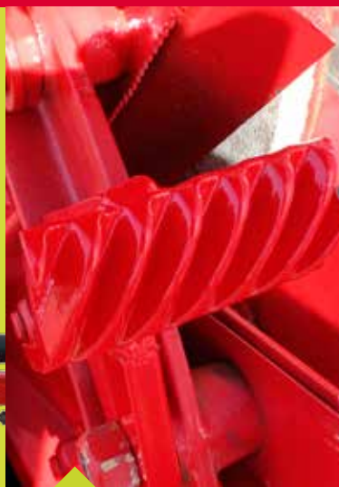
Special paddles For improved kernel crushing.
