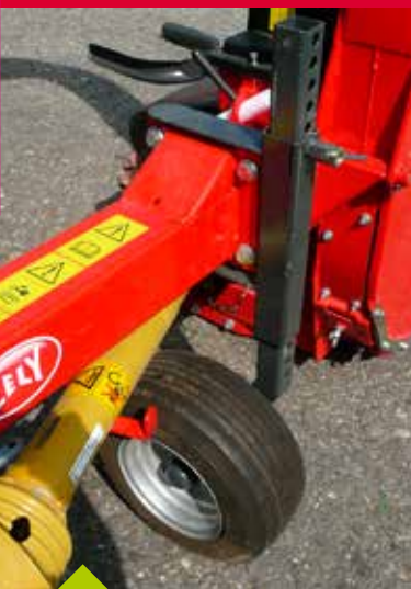
Gaugewheel Pneumatic height adjustable tyres.
