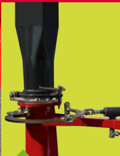
Hydraulic spout adjustment With double acting hydraulic cylinder.
