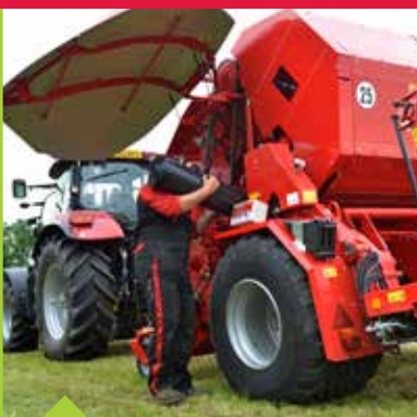
Fourteen film rolls: two on the ring and twelve underneath the guards.
