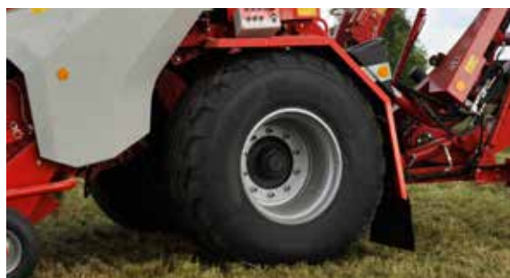
The large tyres ensure minimum ground compaction/ damage, and also give good stability both in the field and in road transport.
