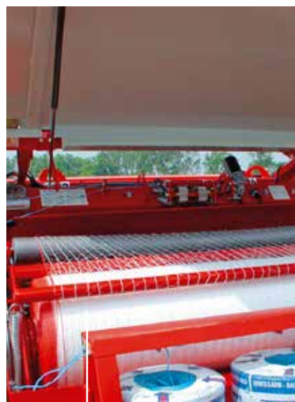
CURVED SPREADING The curved spreading tube conveys the net material up to and just around the edges of the bale.
