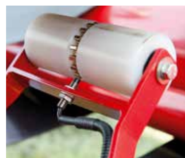
A consistent overlap during the bale rotation being monitored by the sensor-roller.
