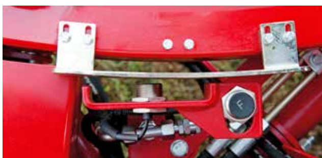
Simple film-break sensor; in the case of a broken film, the bale can be wrapped with the remaining one, or the ring will stop and the broken film can be repaired – programmed from the handset.
