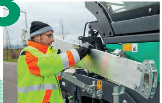
Fix the central beam in position
