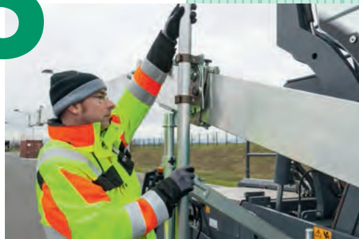
Fit the sensor bracket
