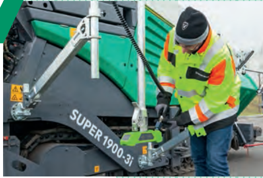
Route cables and connect sensors
