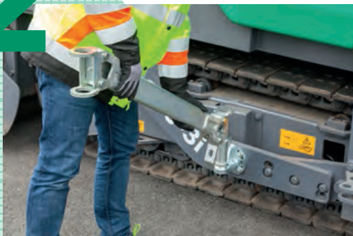
Attach the swivelling arms
