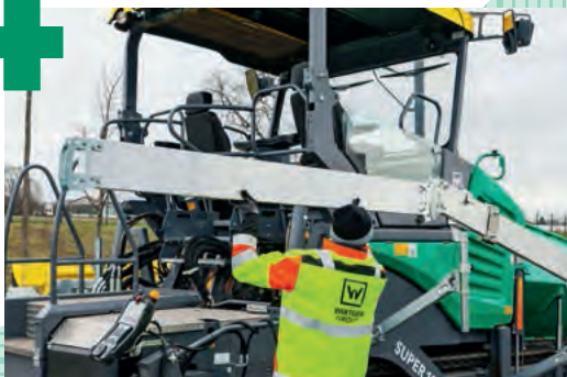
Suspend the extension beam
