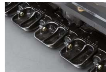
High-durability box construction track shoes
