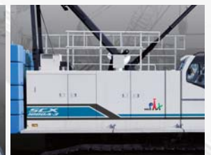
Folding type upper house handrails OPTION
